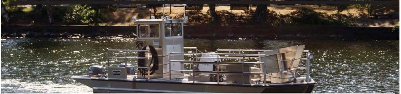
The RRS collects and then transports recovered oil to an offload location.” He added, “As presently configured, the RRS is fully operational in up to 3 foot significant wave height and is able to survive in up to 7 foot waves. Beyond this, it is capable of operating in all weather conditions, with ambient air temperatures ranging from 0 to 105 degrees F, and in water temperatures ranging from 28 to 95 degrees F.”
